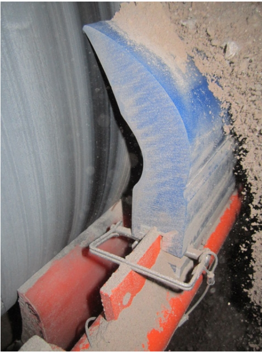
Martin® primary cleaner and a metal tipped secondary Cleaner
