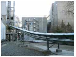
Commissioned in 2002, the Martin® Air Supported Conveyor System at the Coors facility in Golden Colorado incorporates a vertical curve.
