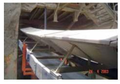
The totally enclosed Martin® Air Supported Conveyor was retrofit onto the structure of an existing belt conveyor.
