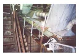
Following the success of the first retrofit, State Line Power Station converted three more conveyors to air-supported, including the SR-1 Conveyor (shown) that carries pulverized coal from the hammer mills to the boiler rooms.
