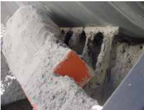
Installed at the five o'clock position near the bottom of the head pulley, Martin® BD Cleaner uses tungsten carbide edges to remove carryback.
