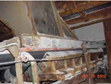
Martin® Self Adjusting Skirting is suitable for use on conveyors with as little as 1.25 inches (32mm) of space on each side of the belt.
