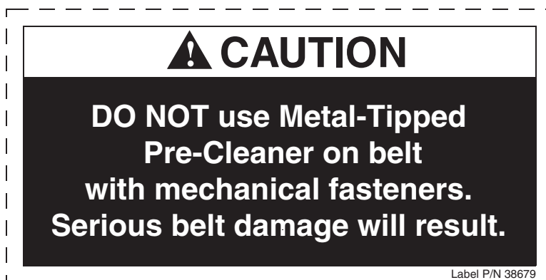
Figure 7. Metal-Tipped Blade Caution Label, P/N 38679
