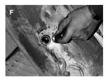
5. If necessary, plug current air inlet fitting on tank with supplied plug (F).
