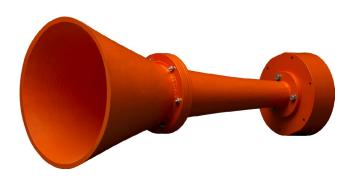
Martin<sup>®</sup> Sonic Horns generate and magnify low-frequency, high-pressure sound waves to cause dry particulate buildup to resonate and fluidize, allowing the material to be removed from the vessel by constant gas flow or gravity. The Martin<sup>®</sup> Sonic Horn 230 Hz produces 147 dB at one meter with a frequency of 230 Hz.
